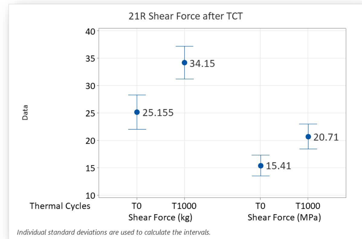
Stable bonding quality before and after thermal cycle test
