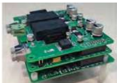
具有自激短路电流健康状态检测功能的 IGBT 驱动电路实物 IGBT drive circuit with self-excited short-circuit current health detection function
