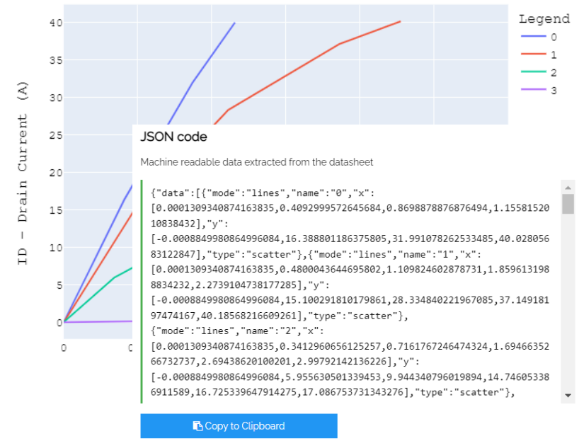
Figure 1: Typical Output Characteristics at 25 °C
