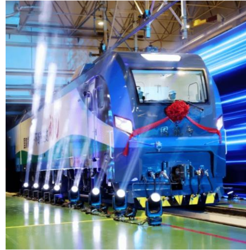
Fig. 2. 10,400kW “GuoNeng”, PMSM direct drive heavy duty electric locomotive
