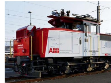
ABB 1.2MW prototype for Swiss Federal Railways with >96% peak efficiency
