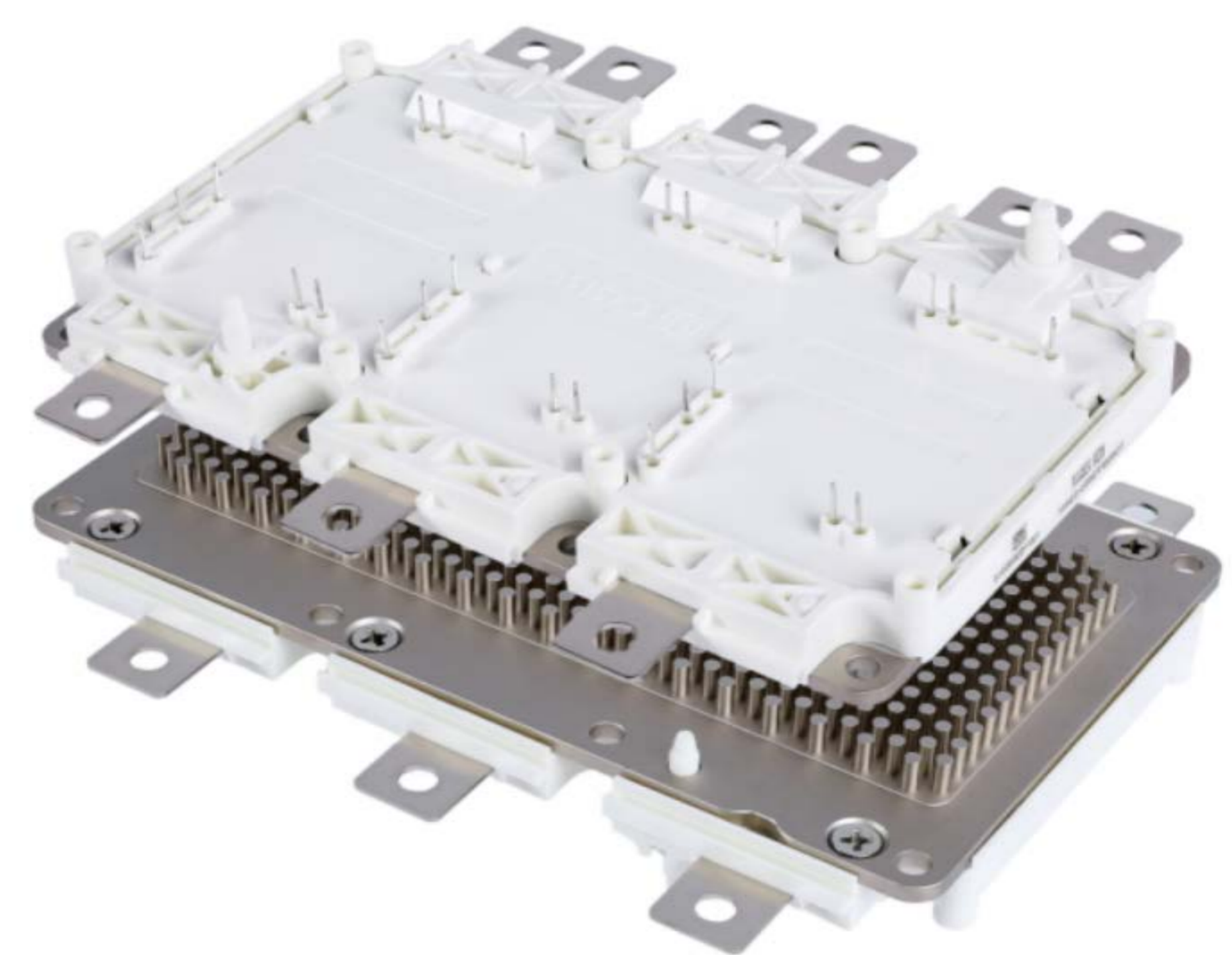
Fig. 6. Demonstrated 600A/1300V S3+ module.
