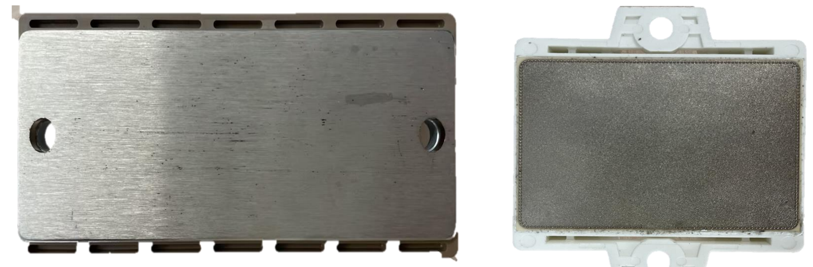
Fig. 3. IGBT module with copper base plate and without copper base plate
