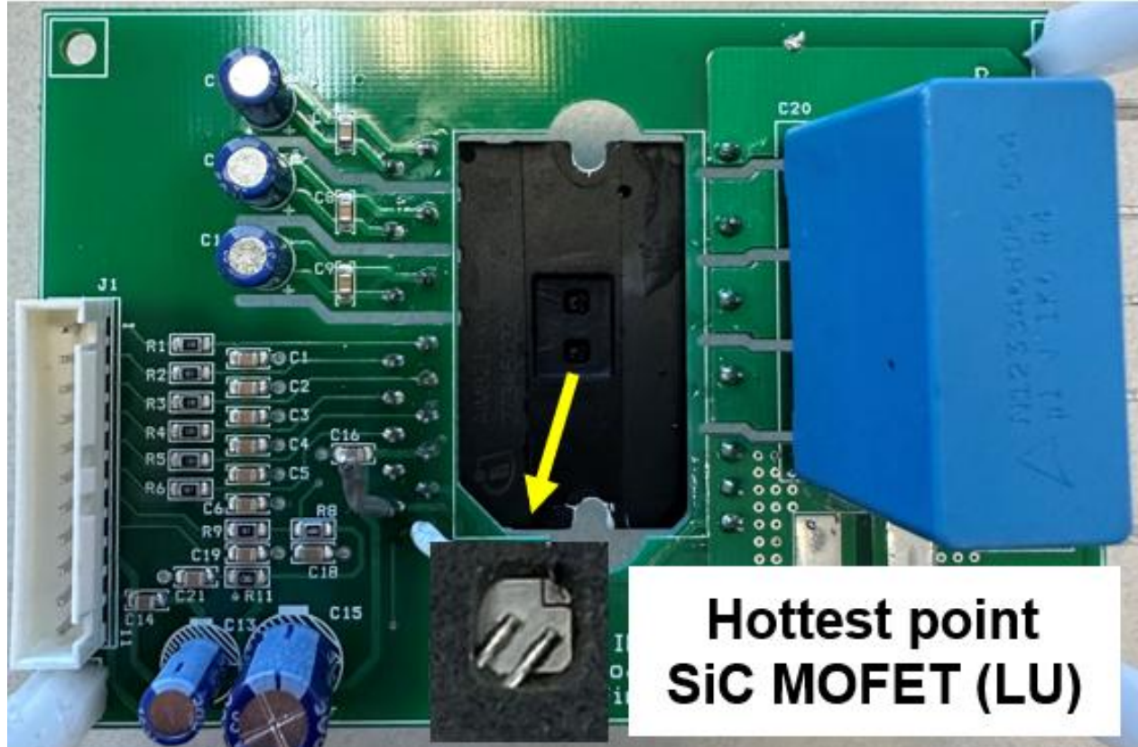
(c) Test board with de-cap sample
